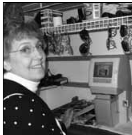
PDG Marian Johnson reads a pair of eyeglasses with the Minot Lions' new lensometer, purchased in 2006. The lens reader reads both eyeglass lenses in about 17 seconds and prints a label.
