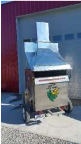
Left Photo Above: Shows the completed Exhaust Hood for the Corn Roaster
